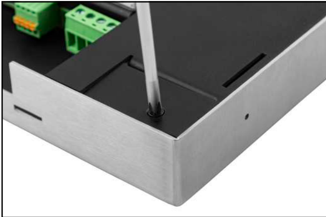
Figure 28. Removing the screw from the access cover
