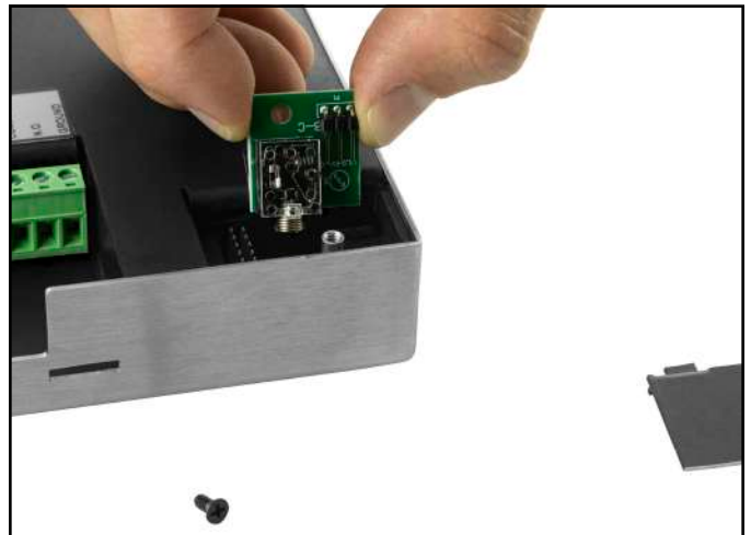
Figure 31. Installing the replacement dual-wire wrist strap jack
