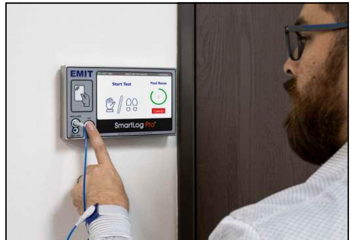
Figure 26. Performing a single-wire wrist strap test
