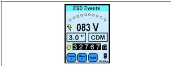
Figure 17. ESD Event voltage display
