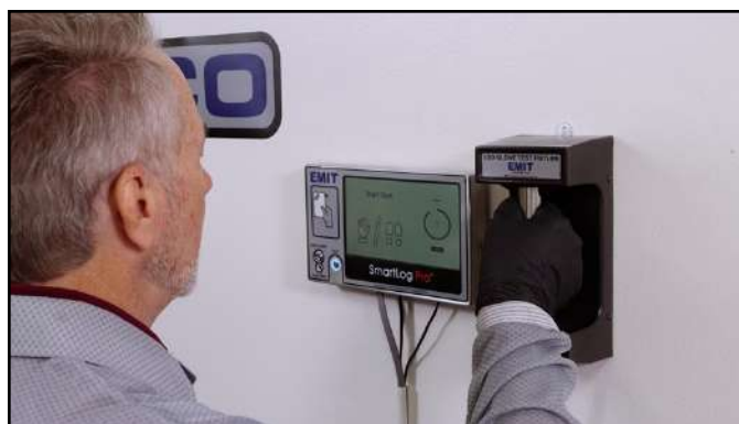
Figure 5. Using the ESD Glove Test Fixture with the SmartLog Pro® 2
