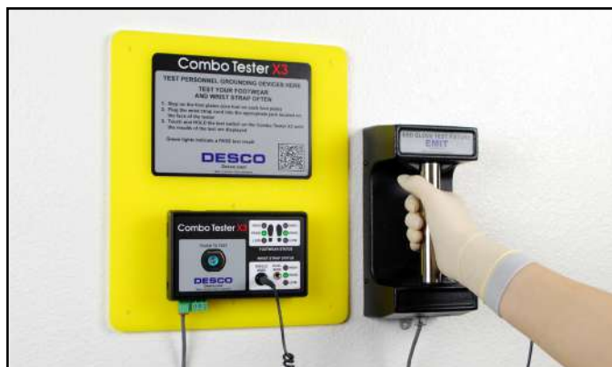
Figure 4. Using the ESD Glove Test Fixture with the Combo Tester X3
