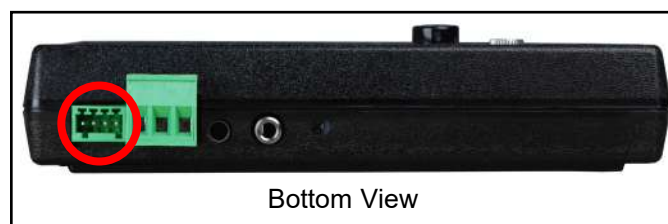
Figure 2. Locating the external test switch port on the Combo Tester X3
