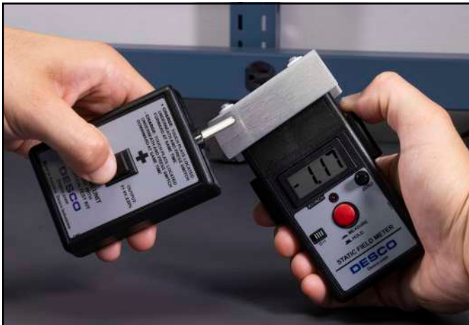
Figure 10. Using the Charger to apply a charge onto the Conductive Plate
