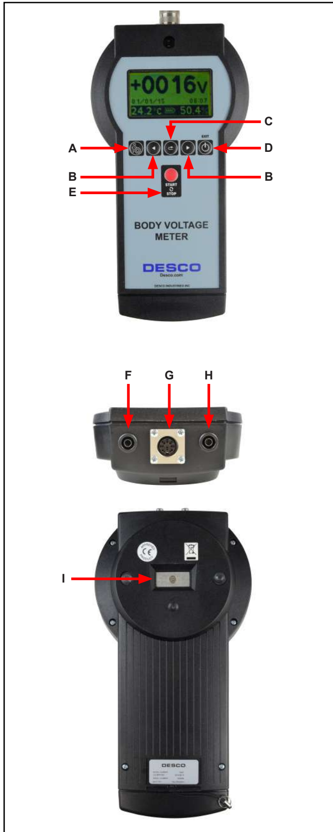
Figure 2. Body Voltage Meter features and components
