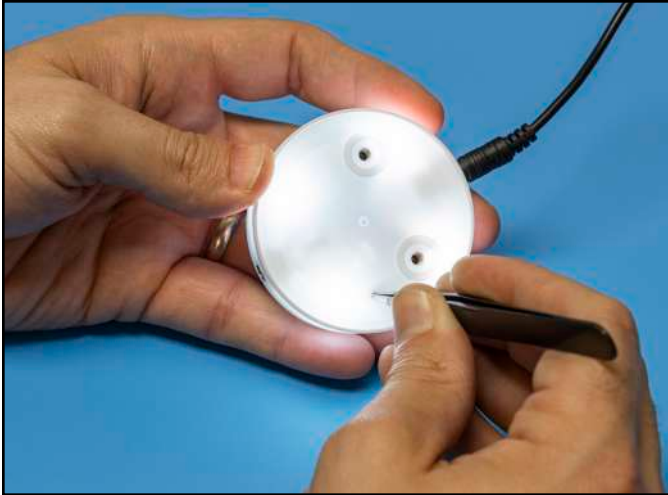
Figure 6. Using the set switch to disable the worksurface monitor circuit
