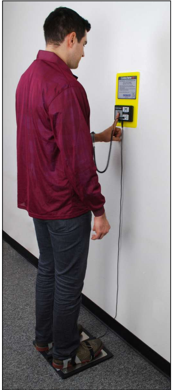
Figure 12. Using the 19270 Combo Tester X3
