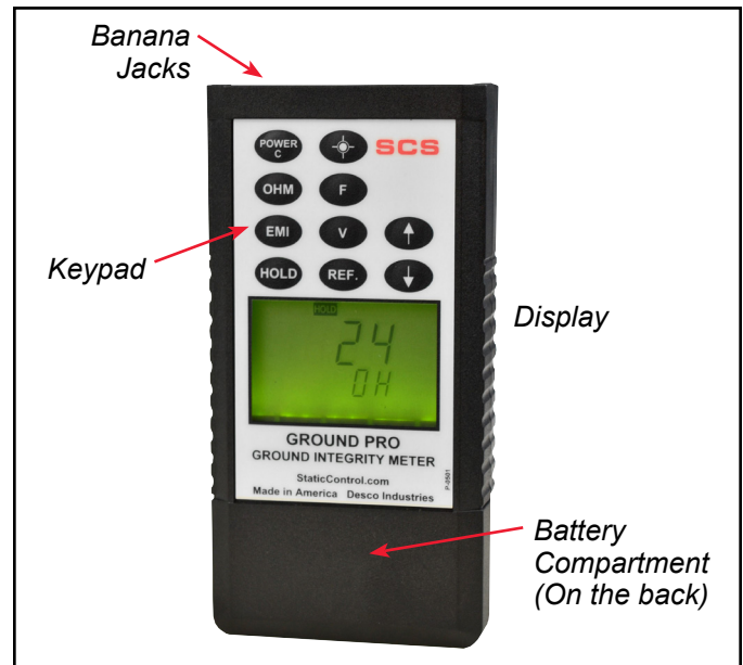
Figure 2. Ground Pro Meter features and components
